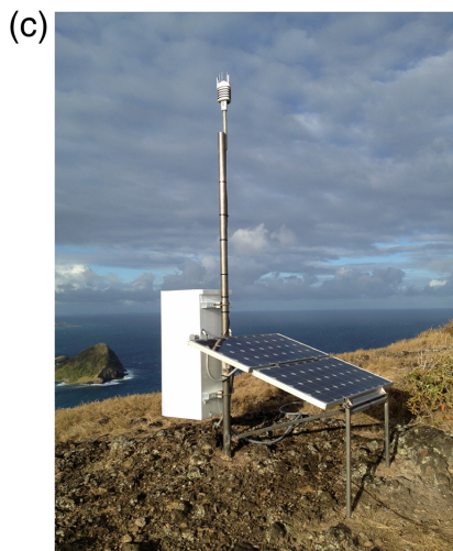
Figure 1. (a) Diagram of typical Network of the Americas (NOTA) permanent Global Navigation Satellite System (GNSS) site configuration. (b) Drilled and braced antenna monument with GNSS antenna. (c) Additional components of this installation include an enclosure for GNSS receiver and communications and power devices, solar panels, and a meteorological instrumentation package. Image credit: UNAVCO Inc. The color version of this figure is available only in the electronic edition.
