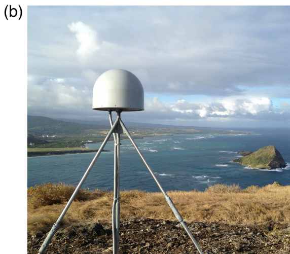
Figure 1. (a) Diagram of typical Network of the Americas (NOTA) permanent Global Navigation Satellite System (GNSS) site configuration. (b) Drilled and braced antenna monument with GNSS antenna. (c) Additional components of this installation include an enclosure for GNSS receiver and communications and power devices, solar panels, and a meteorological instrumentation package. Image credit: UNAVCO Inc. The color version of this figure is available only in the electronic edition.
