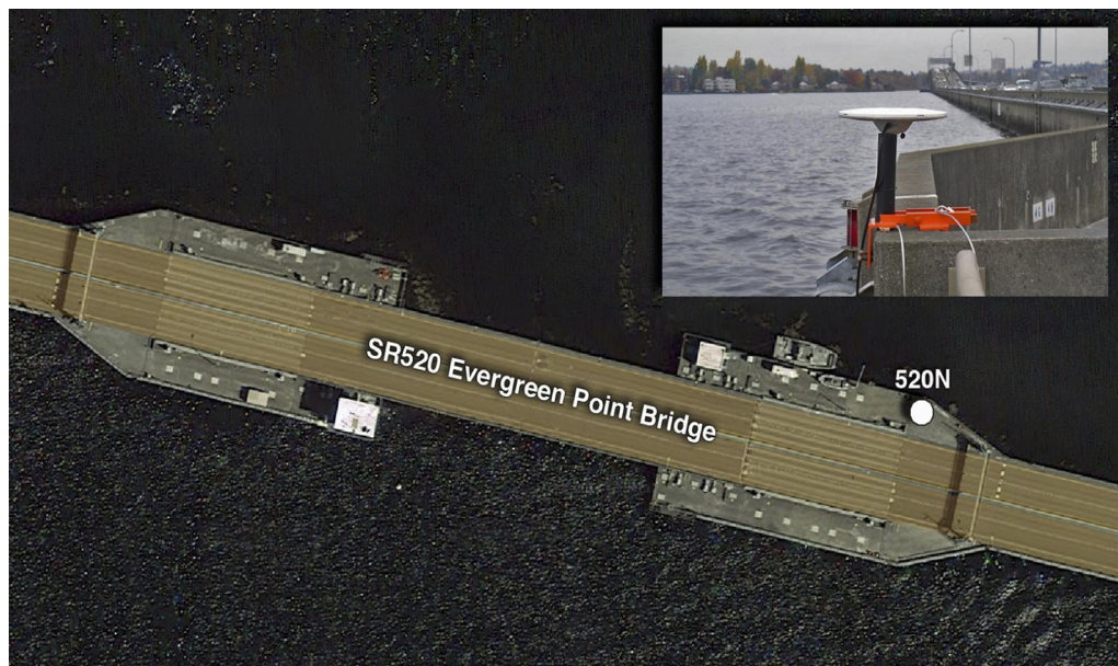
Fig. 1. (Color) Aerial view of the Evergreen Point Floating Bridge (SR520) across Lake Washington; GPS receiver 520N was installed midway across the 2.3-km floating section in late 2011 and operated through December 2012 (Imagery © 2015 Google, Landsat, USDA Farm Service Agency, Map data; inset image by Rex M. Flake)
