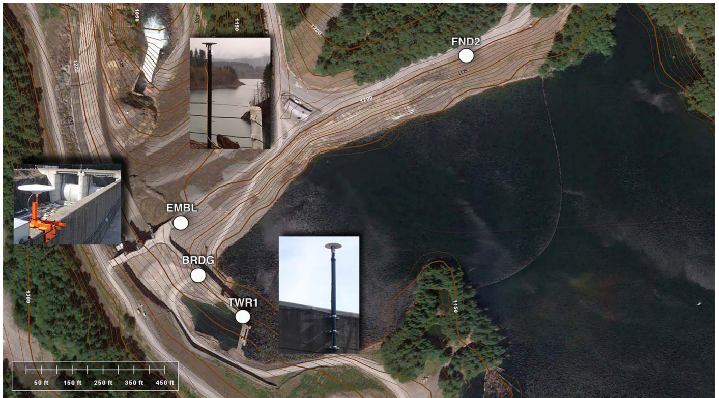
Fig. 3. (Color) Aerial view of the Howard A. Hanson Dam, located in the Green River west of Tacoma, Washington; only GPS stations whose data are shown in Fig. 8 are shown here; a total of 14 were installed (Imagery © 2015 Google, Landsat, USDA Farm Service Agency, Map data; inset images by Rex M. Flake)
