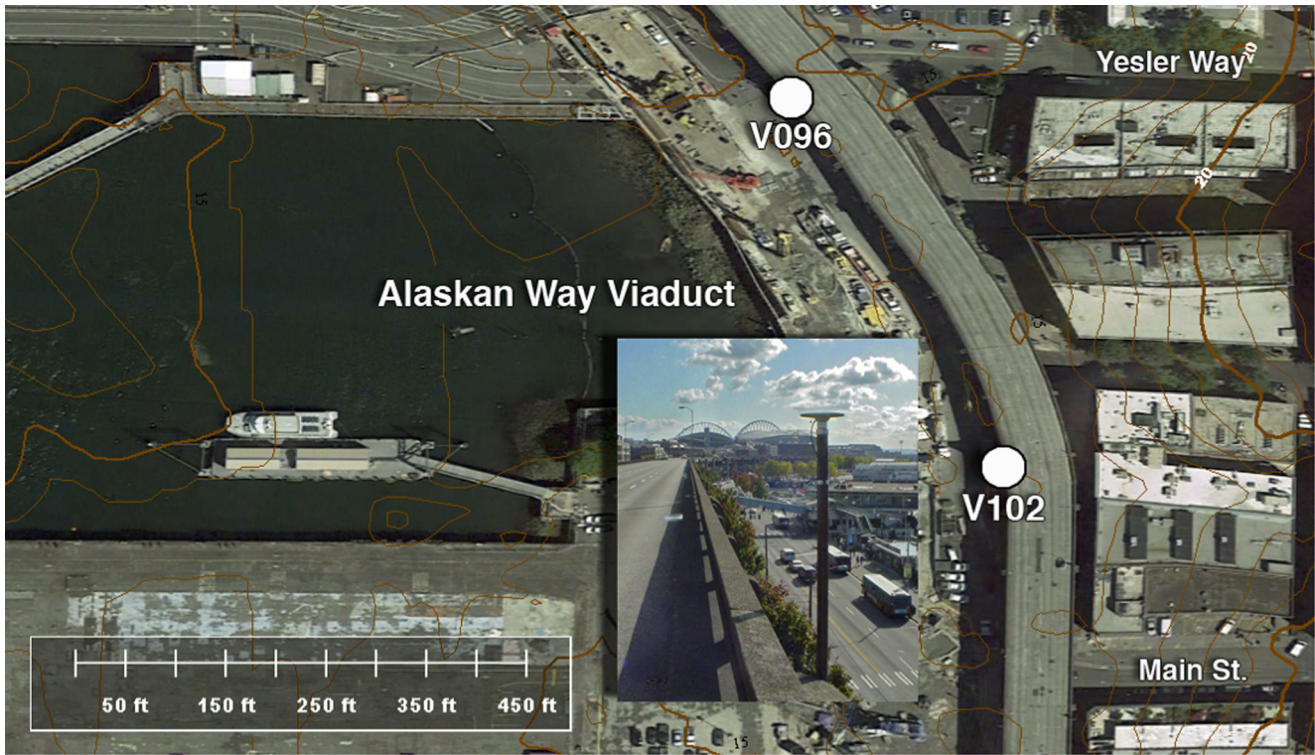
Fig. 2. (Color) Aerial view of the 6-lane elevated Alaskan Way Viaduct (SR99) through downtown Seattle. Antennas of GPS stations V096 and V102 were mounted on 4-m schedule-15 steel pipe to minimize disruption of sky view by freeway traffic (Imagery © 2015 Google, Landsat, USDA Farm Service Agency, Map data; inset image by Rex M. Flake)
